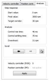
As can be seen by the reduced control settling time and the reduced overshoot in the example shown here, following optimisation of the speed control gain to value 5 the drive has a significantly more dynamic performance.
